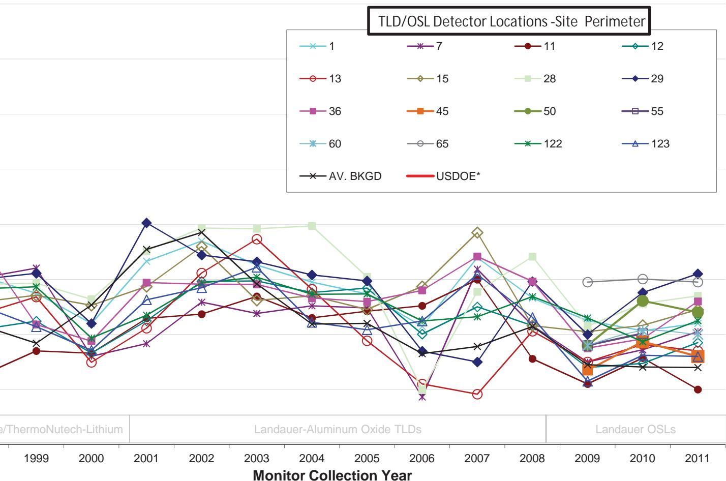
**FIGURE 9: EXTERNAL GAMMA RADIATION DOSE RATES AT IWCS PERIMETER**
